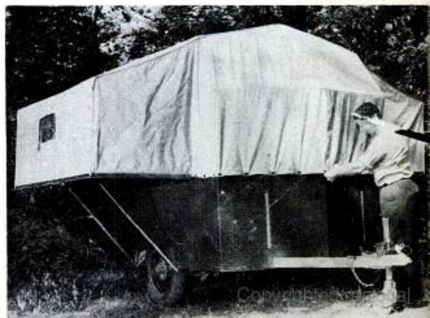
Above, pipe framework swings upward from trailer body to support tent roof like covered wagon. Steps under body keep trailer from tipping. Below, Jim Kendall buttons canvas to row of regular curtain fasteners which are added to front of trailer
